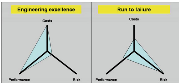
Fig. 1 Extremes in the cost/risk/performance balance, adapted from Yorkshire electricity (Wijnia and Huisma 2007)
